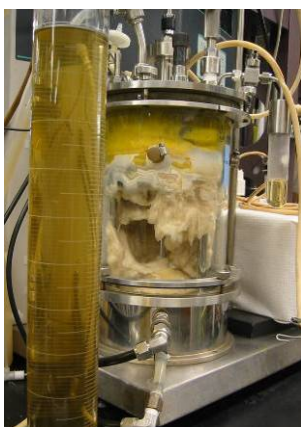
Figure 3.10. Clarified effluent and bioreactor vessel filled with biomass after fungal cultivation in thin stillage (5 L) for 7 days with 0.4-vvm aeration.
