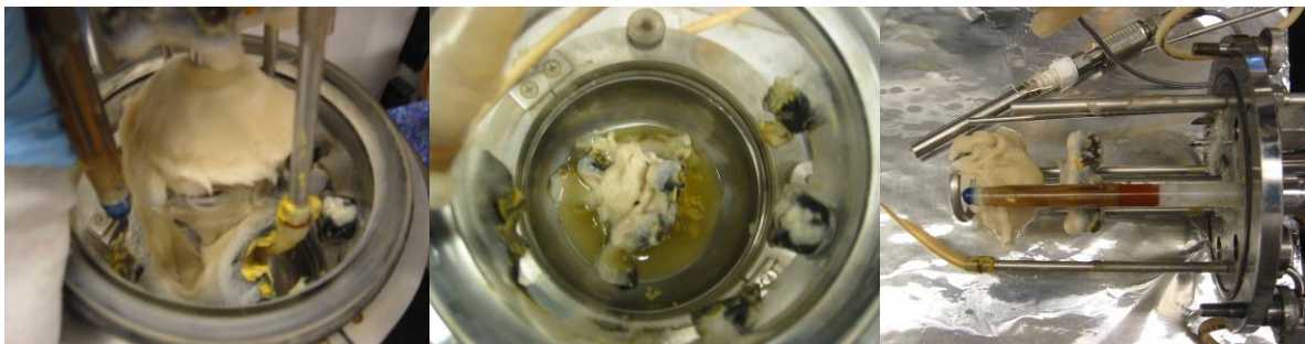
Figure 3. Fungal biomass harvested from the reactor on day 7. Views of fungal mycelia, from left to right, as the head plate was lifted from the reactor, inside the vessel, and on the agitator shaft.
